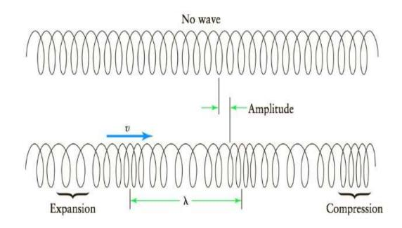
Another example of Longitudinal Waves in fluids (liquids and gases) is shown, notice the compression and expansion (refraction) areas.
